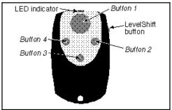
4 are the smaller buttons to the right, below and left of button 1. The LevelShift button on the side permits you to select channels 5–12 with the same four buttons.
